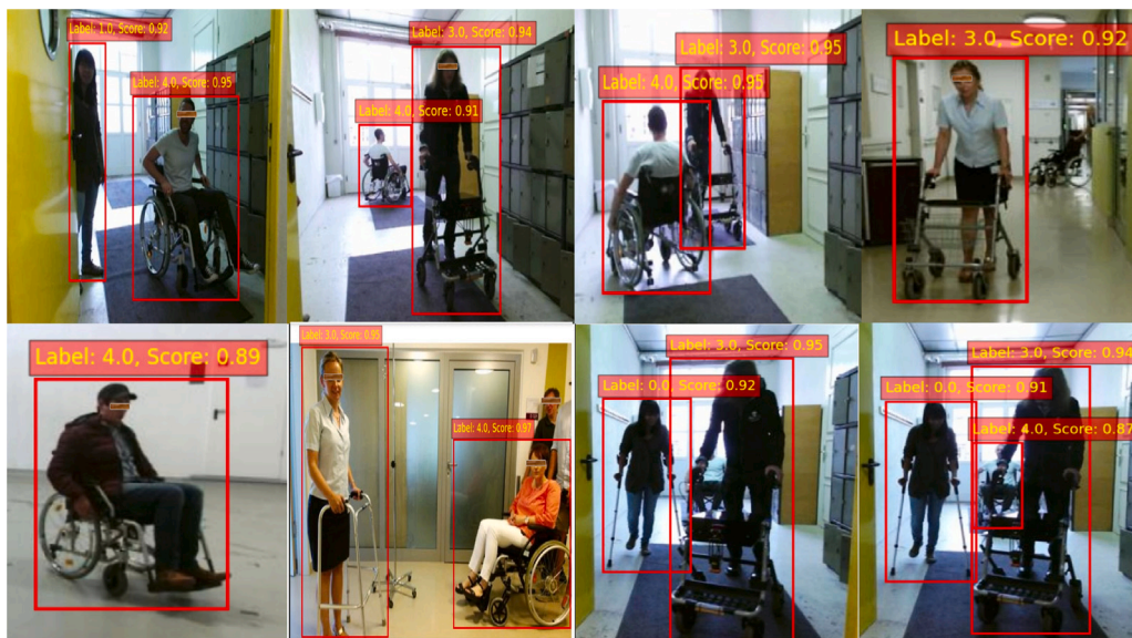
Fig. 11. Detection results of mobility disabilities with the hybrid YOLO v10 with the RCNN framework: 'crutches=0', 'person=1', 'push_wheelchair=2', 'walking_frame=3', 'wheelchair=4'.
